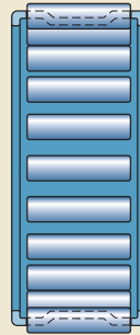
Sheet steel cage of the radial bearing
